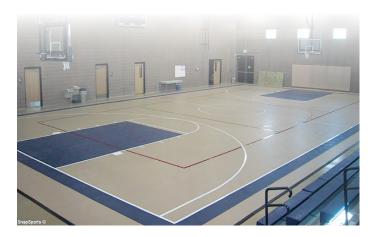
**FLOORS CONTAIN MERCURY:** Rubber-like polyurethane floors using 1,000 to 2,000 parts per million (ppm) of phenyl mercuric acetate (PMA) catalyst have been installed in school multipurpose rooms, gyms, cafeterias, auditoriums, stages, and indoor and outdoor tracks since the 1960s.
