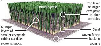
This graphic shows a typical multilayered structure. Plastic grass "blades" (ingredients historically included lead) attach to a fabric backing, separated by an "infill" (usually the tire "crumbs," and sometimes sand). Below them are stones through which drainage pipes go. The infill provides "give." From cdn3.vox-cdn.com/assets/4335789/turfjgraphic.jpg.
